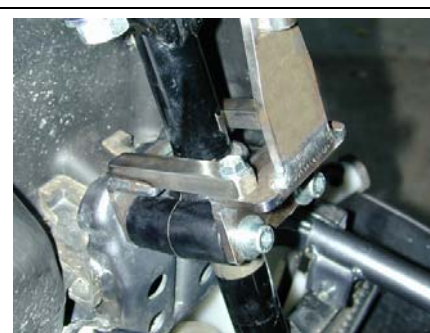
Frame bracket installed
