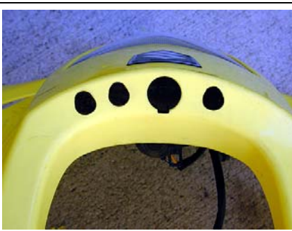
Finished gauge holes
