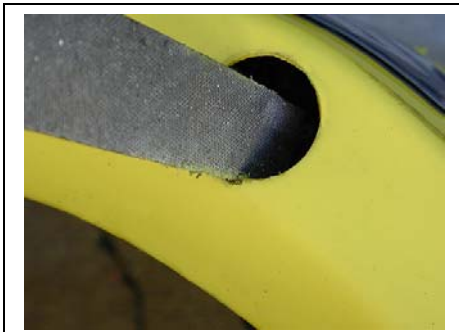
Notching the ignition hole with file
