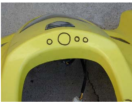
Marking where the gauges will go
