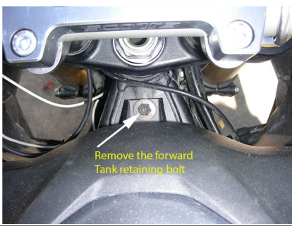
Remove the forward tank bolt
