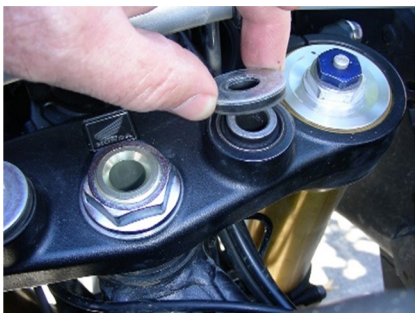
Retain stock rubber/washer between the Sub assembly and triple clamp
