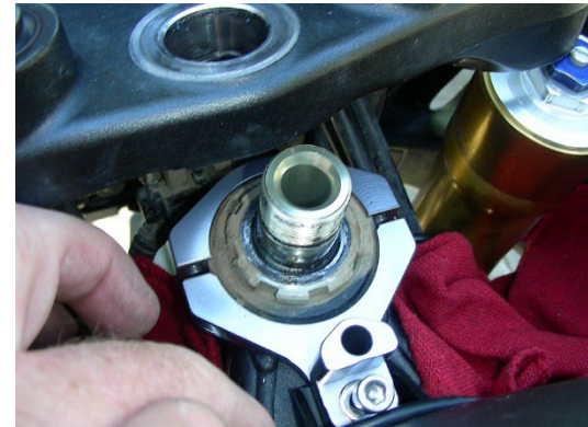
Lift the triple clamp up just high enough to install the new frame bracket.
