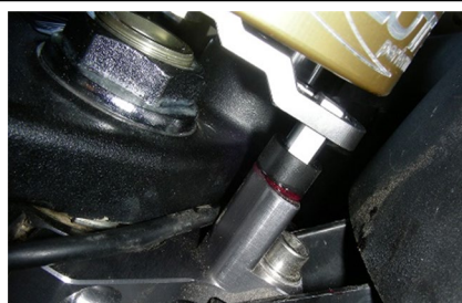
Tower pin greased & installed correctly
