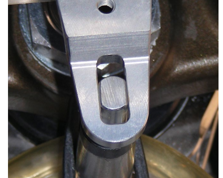
This shows the tower pin centered in the middle of the slot of the link arm. If yours is not centered you may have the lower perches reversed and need to correct the problem or you could damage your stabilizer internally.
